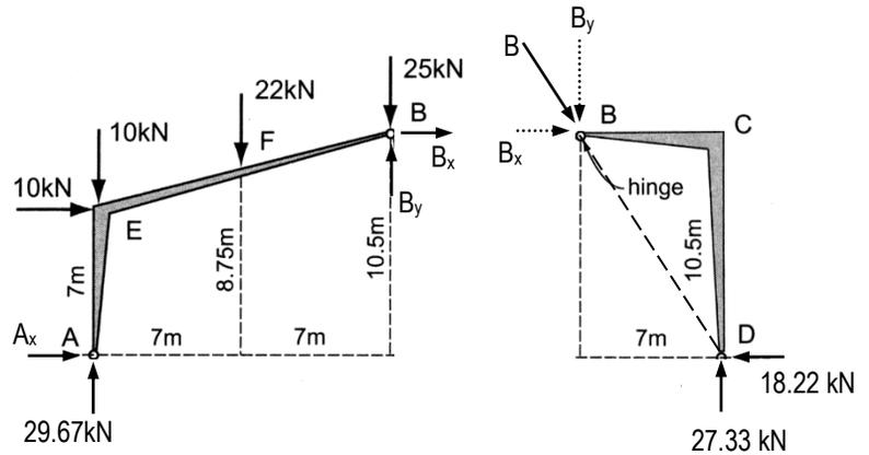
So the horizontal reaction force at B pushes to the left on the left FBD and to the right (opposite) on the right FBD, while the vertical reaction force at B pushes up on the left FBD and down (opposite) on the right FBD.
