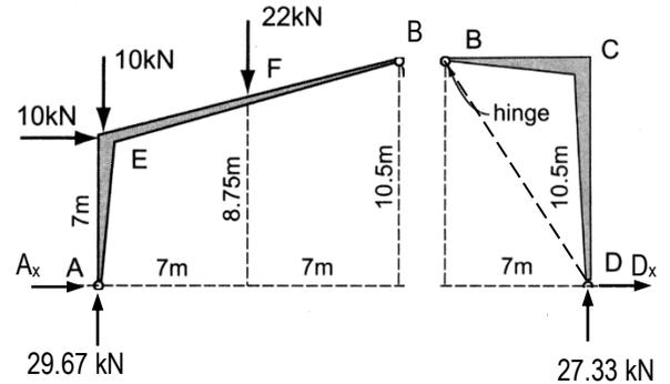
We can find  $D_x$  (which must be pointing into D like  $D_y$  is) with similar triangles:
