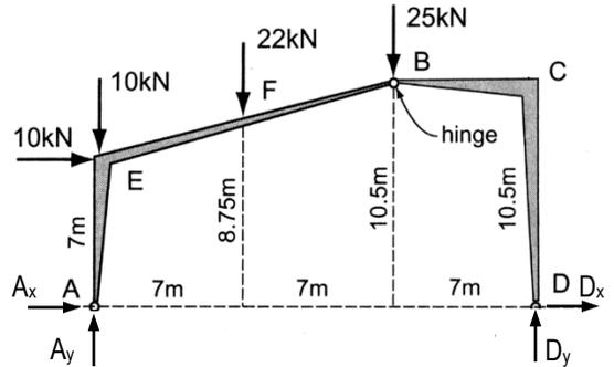
Draw the FBD's for the parts, and wait to put on the 25 kN load at B because it can only go on one FBD. We'll also wait to draw the connection force components at B:
