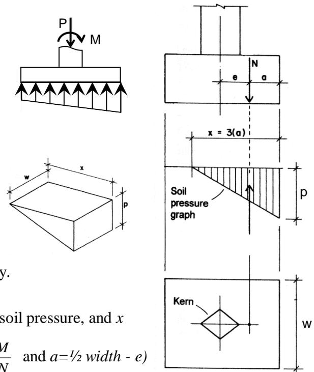
If the contact is gone, the maximum pressure can be determined knowing that the volume of the *pressure wedge* has to equal the column load, and the centroid of the *pressure wedge* coincides with the effective eccentricity.
