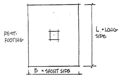
6) Check transfer of load from column to footing: ACI 16.3
