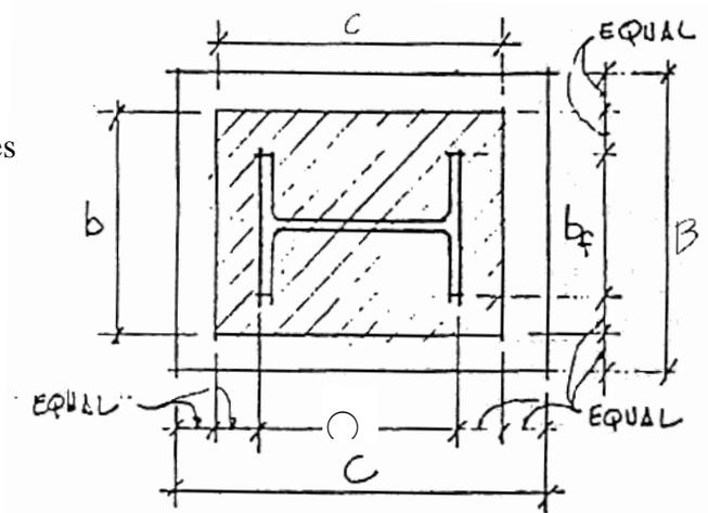
$$b = b_f + \frac{(B - b_f)}{2} \text{ where } b_f \text{ is the width of column flange and } B \text{ is base plate side}$$
