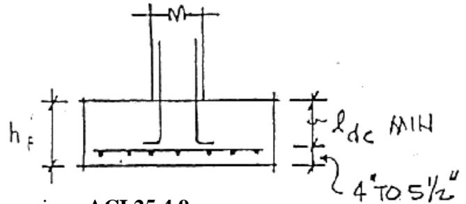
d) Check dowel embedment into footing for compression: **ACI 25.4.9**
