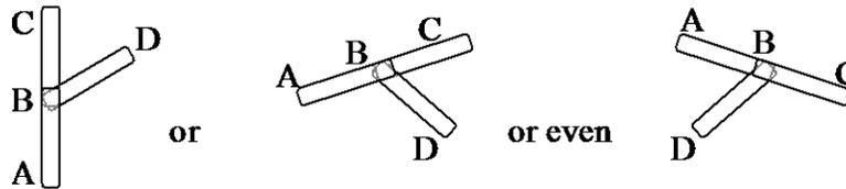
$F_{AB}$  and  $F_{BC}$  have to be equal, and  $F_{BD}$  has to have zero force.
