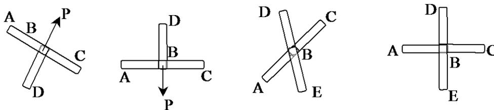
$F_{AB}$  has to equal  $F_{BC}$ , and [ $F_{BD}$  has to equal  $P$ ] or [ $F_{BD}$  has to equal  $F_{BE}$ ]
