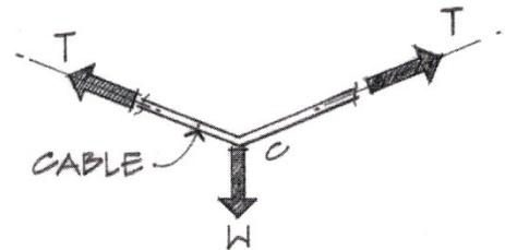
The forces anywhere in a *straight segment* can be resolved into x and y components of  $T_x = T \cos \theta$  and  $T_y = T \sin \theta$ .
