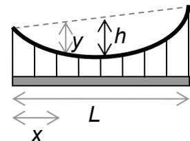
where  $y$  is the vertical distance from the straight line from cable start to end
