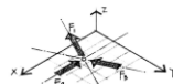
Coplanar, concurrent—All forces intersect at a common point and lie in the same plane. Figure 2.17(d) Particle or rigid body.
