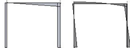
**4.4 & 5** A fully fixed single-bay frame has a span of 36 ft and a height of 13.5 ft and carries a uniform loading of 4.2 k/ft on the beam. The moment of inertia of the beams is roughly  $2/3$  of the moment of inertia of the column. The results provided are below and the diagrams are on the following page:
