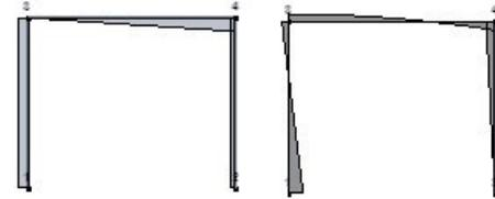
**4.3** For the frame of problem 4.1, replace the pin support with a fixed support and use an approximate method of analysis to draw the shear and moment diagrams (from the formulas provided). Indicate numerical values.
