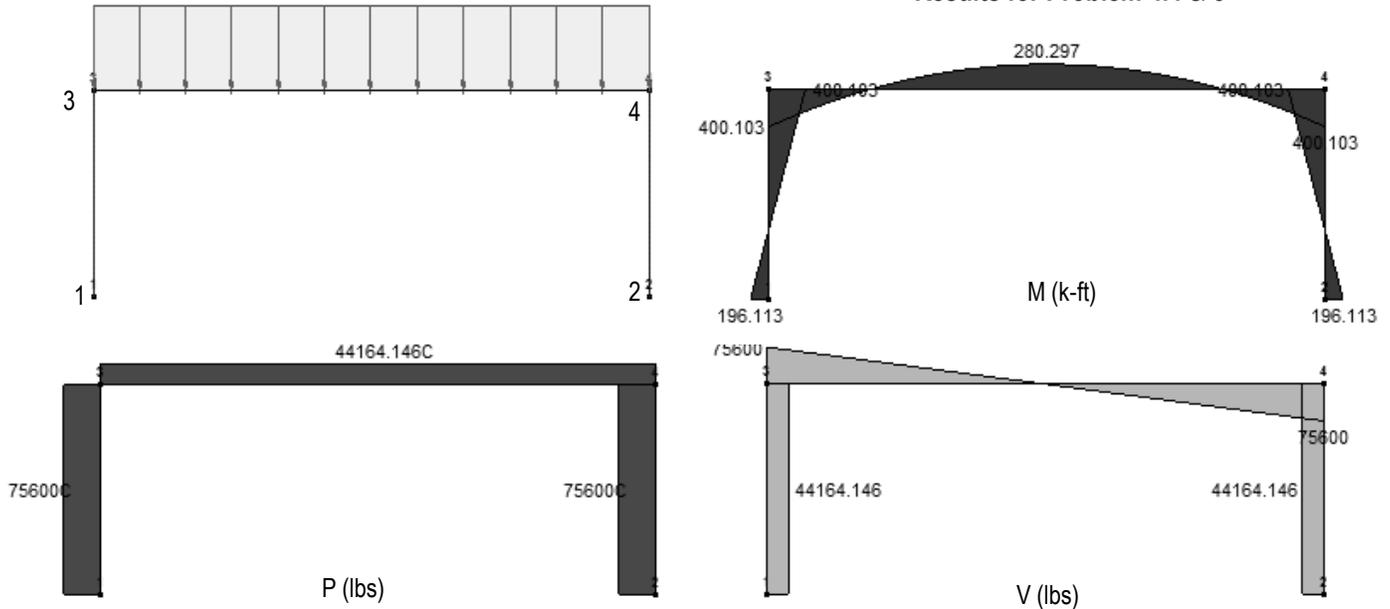
Calculate the maximum stress at the ends of both columns from combined bending (M/S) and compression stresses (P/A).
