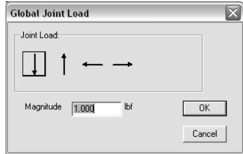
Multiframe2D will automatically generate a grouping called a Load Case named Load Case 1 when a load is created. All additional loads will be added to this load case unless a new load case is defined (Add case under the Case menu).
