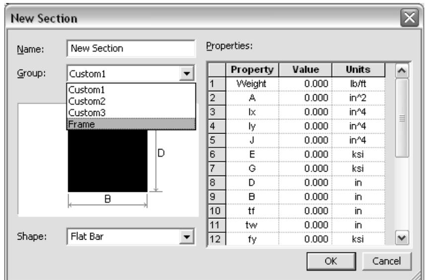
Table values 1-9 must have values for a Flat Bar, but not all are used for every analysis. A recommendation is to put the value of 1 for those properties you don't know or care about. Properties like  $t_f$ ,  $t_w$ , etc. refer to wide flange sections.
