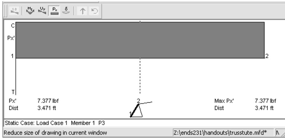
13. The Data window (D) allows you to view all data “entered” for the geometry, sections and loading. These values can be edited.
