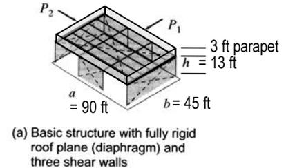
2. For the shear wall on the long side ( $R_3$ ) of the building in Problem 1, determine the overturning moment.
