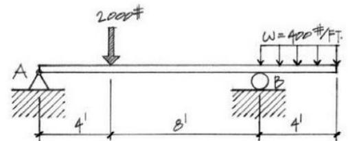
**\*Use superpositioning with the Beam Diagrams and Formulas to get support reactions to construct the V & M diagrams.**
